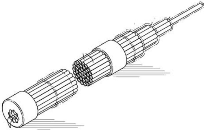
Figure 3: Waveguide Vibration Sensor Reflection Elimination Through Incoherent Reflection
