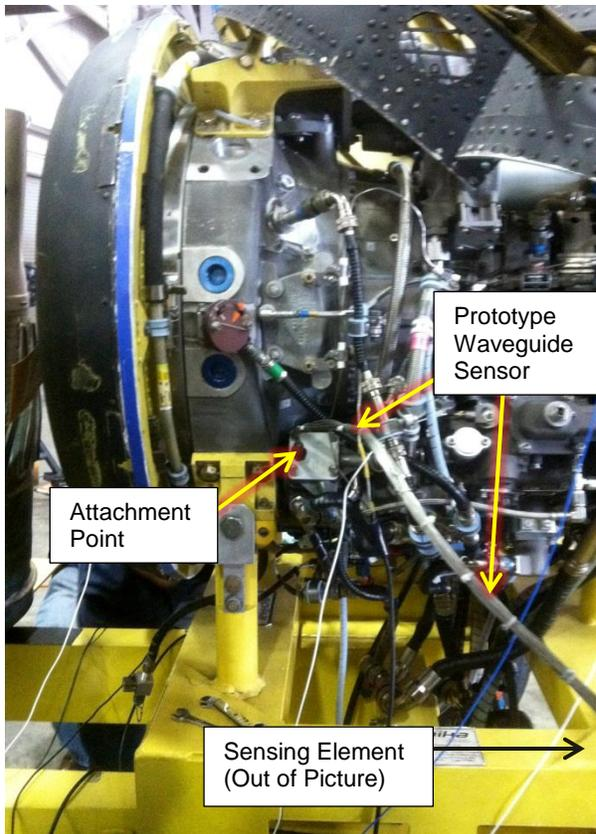
Figure 5: Waveguide Sensor Mounted on Chinook T55 Engine
