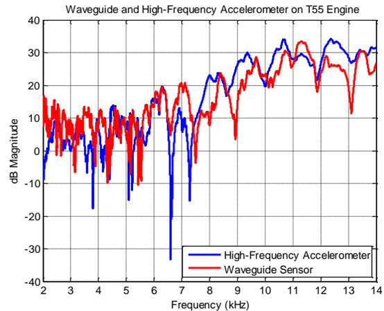
Figure 6: Comparison of Waveguide and High-Frequency Accelerometer on Chinook T55 Engine
