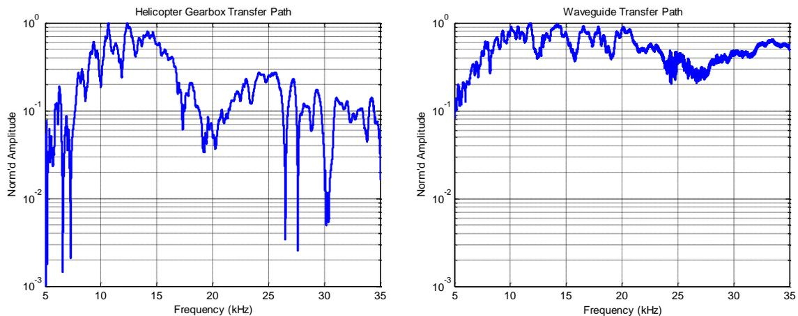
Figure 9: Helicopter Gearbox Transfer Path (Left Trace) Has Large Dynamic Range and Substantially Alters the Vibration Signal; Waveguide Sensor Transfer Path (Right Trace) Has Narrow Dynamic Range and Does Not Significantly Alter the Vibration Signal.
