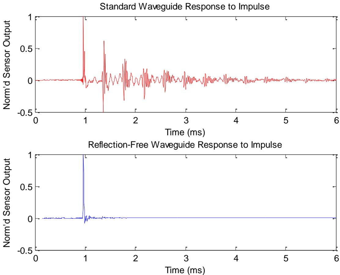
Figure 2: Design of Passive Waveguide to Eliminates Reflections (Bottom), Enabling True Broadband Response, Compared to Uncompensated Waveguide (Top)
