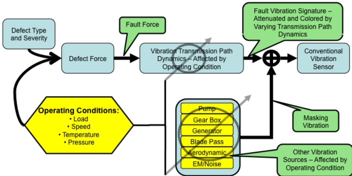
Figure 7: Schematic Showing Operating-Condition Sources for Change in Vibration Transfer Path which Affect Measured Vibration Amplitude
