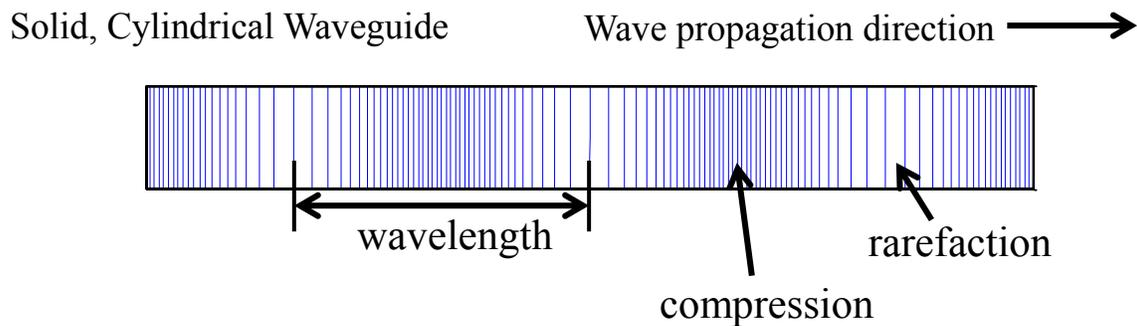
Figure 1: Stress-Wave Propagation Through a Cylindrical Waveguide
