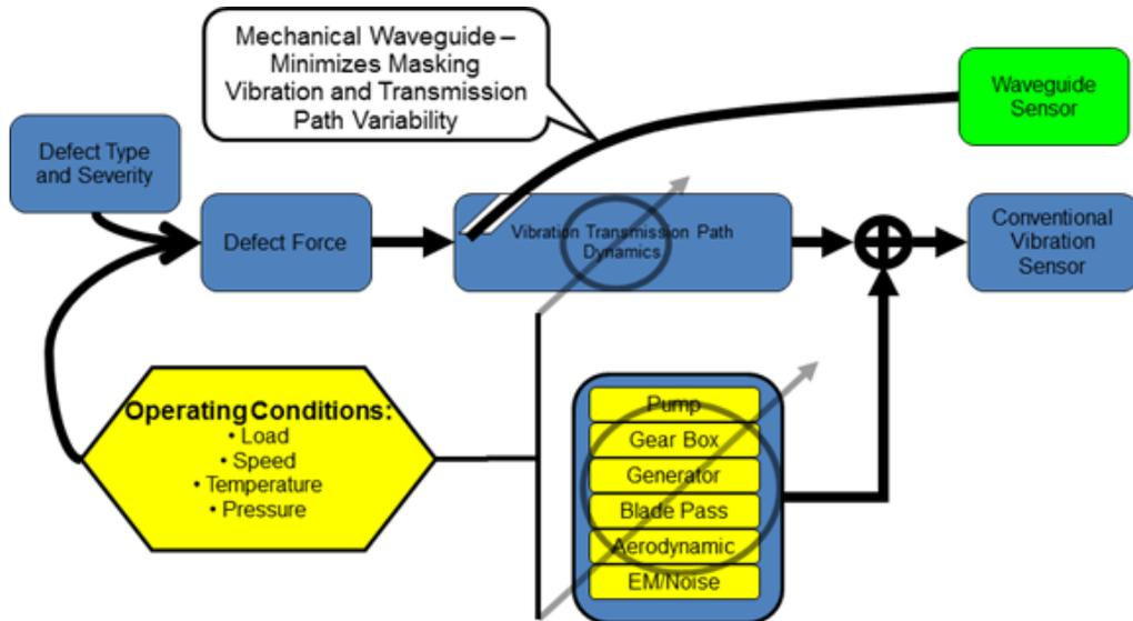
Figure 8: Schematic Showing Operating-Condition Sources for Change in Vibration Transfer Path which Affect Measured Vibration Amplitude
