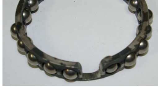
Figure 2. Removal of One Bearing Element
