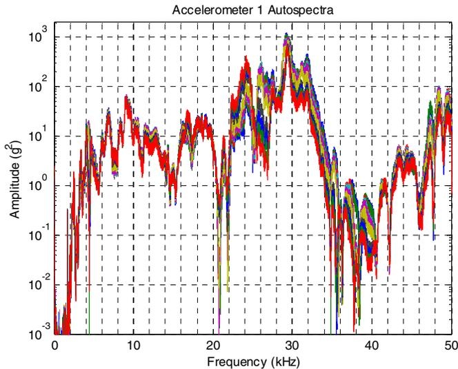
Figure 2. Repeatability of an individual accelerometer near its mounted resonance
