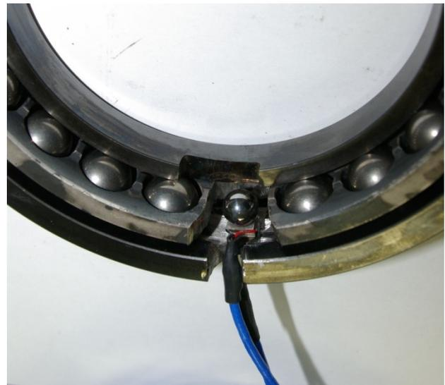
Figure 5. Reaction-mass shaker with force-measurement sensor placed in bearing for defect transfer path measurement.
