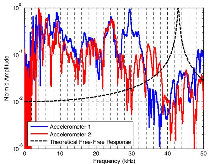
Figure 1. Mounted accelerometer resonance dependent on structure and mounting conditions
