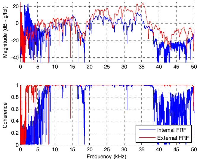
Figure 6. Internal and external FRFs measured on Apache IGB
