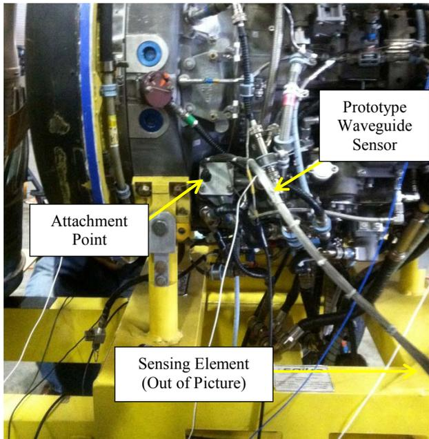
Figure 8. Prototype broadband waveguide vibration sensor mounted to Chinook T55 turbine engine.
