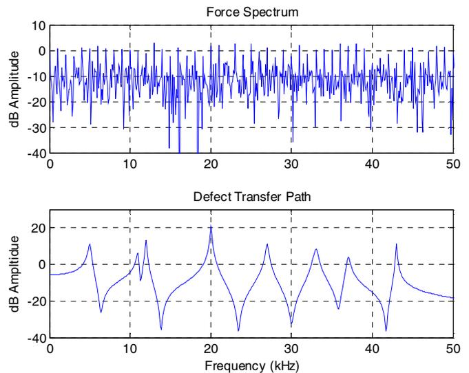
Figure 3. Synthetic force input spectrum (top) and FRF (bottom)
