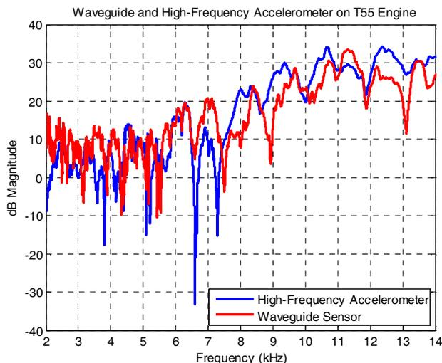
Figure 9. Transfer path comparison between high-frequency accelerometer and broadband waveguide.
