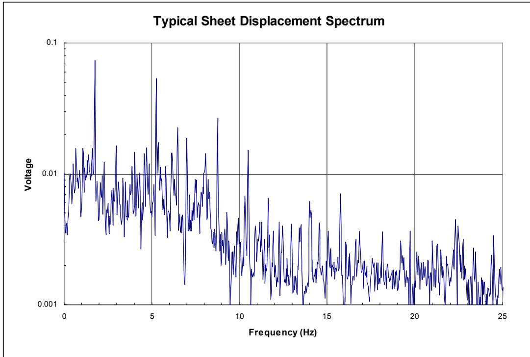
Figure 7: Out-of-plane sheet motion above air knife.
